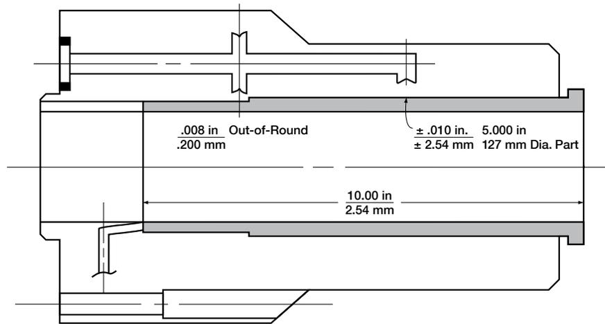
Conform-A-Chucks and Conform-A-Arbors are a revolutionary new concept in hydraulic holding devices. Conceived, developed and patented by Hydra-Lock Corporation, Conform-A-Chucks and Conform-A-Arbors are truly the **PROBLEM SOLVERS FOR THIN-WALLED PARTS.**
